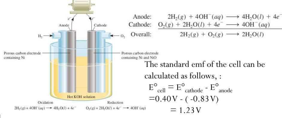
A hydrogen-oxygen fuel cell.
