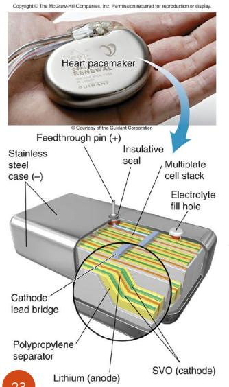
The primary lithium battery is widely used in watches, implanted medical devices, and remote-control devices.
