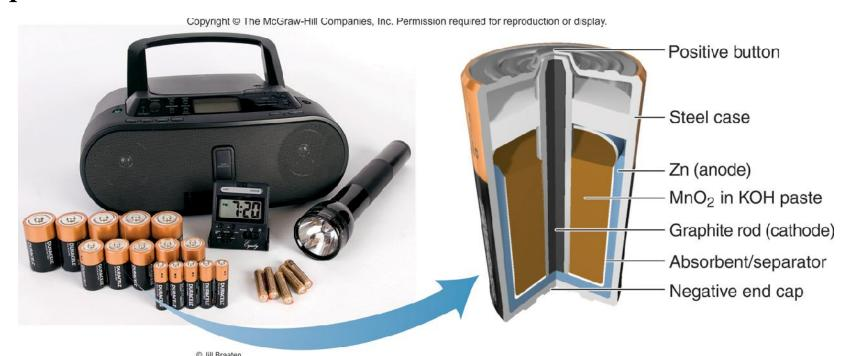
Anode (oxidation):  $Zn(s) + 2OH^{-}(aq) \rightarrow ZnO(s) + H_{2}O(l) + 2e^{-}$ Cathode (reduction):  $MnO_{2}(s) + 2H_{2}O(l) + 2e^{-} \rightarrow Mn(OH)_{2}(s) + 2OH(aq)$ Overall (cell) reaction:
