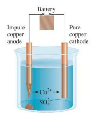
Anode:  $Cu(s) \longrightarrow Cu^{2+}(aq) + 2e^{-}$ Cathode:  $Cu^{2+}(aq) + 2e^{-} \longrightarrow Cu(s)$
