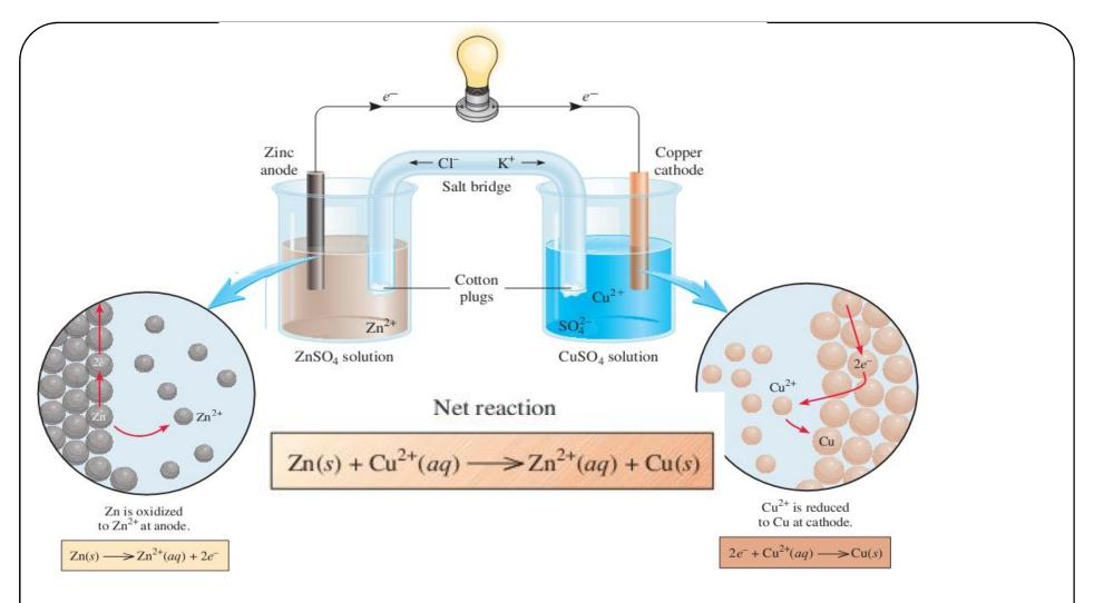
A galvanic cell. The salt bridge (an inverted U tube) containing a KCl solution provides an electrically conducting medium between two solutions. The openings of the U tube are loosely plugged with cotton balls to prevent the KCl solution from flowing into the containers while allowing the anions and cations to move across. The lightbulb is lit as ctrons l ow externally from the Zn electrode (anode) to the Cu electrode (cathode).
